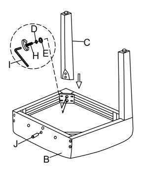
Take the Allen Key, and turn the bolts until the legs are secure. DO NOT TIGHTEN COMPLETELY. Stop when you feel you are adding force to tighten the bolt.
