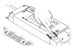
2. If setting WAV Smart Receiver / Power Supply up for the first time, clear the memory by pressing and holding the "Prog" button until the lights blink twice.
