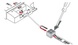
4. Use #1 Phillips to loosen the 4 terminal screws on 8MM-EZ Connector. Peel 1/2" of the adhesive protector from back of LED tape light, and scrape waterproof coating, insert into connector, evenly tighten screws. Insert wires from WAV Smart Receiver / Power Supply into terminals, Red wire to (+ or WW) side of tape, Black wire to (- or CW) side of tape; tighten screws.
