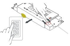
5. Plug WAV Smart Receiver / Power Supply into 120V receptacle and pair to Controller.
