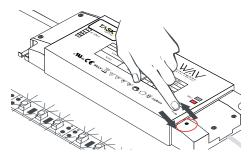
2. If setting WAV Smart Receiver / Power Supply up for the first time, clear the memory by pressing and holding the "Prog" button until the lights blink twice.
