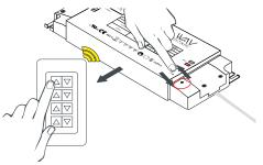
5. Plug WAV Smart Receiver / Power Supply into 120V receptacle and pair to Controller.
