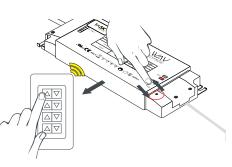
3. Very quickly, click and release the "Prog" button and, within 5 seconds, quickly click and release the "On Light Bulb" button on the Controller. When lights blink once, Controller and Receiver are paired.
