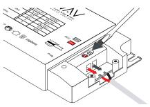
3. Insert one end of stripped wires into WAV Smart Receiver LED Terminals, Red wire to (WW+) and Black wire to (CW-) terminals. Tighten screws.
