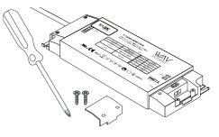
2. Use #2 Phillips to loosen screw and remove cover from WAV Smart Receiver / Power Supply. Use the flat head from the multi-bit screwdriver to loosen one terminal marked (CW-) and one marked (WW+).
