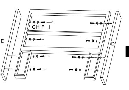
Attached Side Panel (D) (E) to the Headboard (A) use Bolt (F), Lock Washer (H) and Flat Washer (G). Turn the Allen Wrench (I) in Bolt (F).
