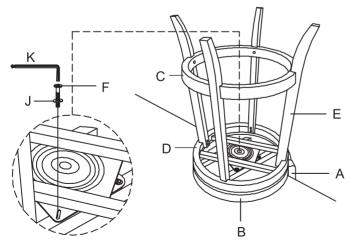
Stand chair up on an even surface and check that it is balanced. If there is a slight wobble, apply downward pressure in the corner where a leg is uneven. Keeping pressure in that corner, tighten all bolts. If balanced, apply downward pressure evenly in the center and tighten all bolts. Do not over-tighten beyond hole depth.
