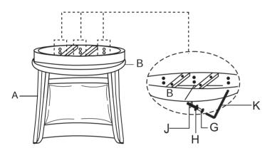
3 Keep the Backrest (A) and Cushion Seat (B) inverted on a stable raised surface. Attached the Swivel Plate located on the Apron With Swivel Plate (D) to the Cushion Seat (B) using Bolt (F), Flat Washer (J) with Allen Wrench (K). Turn the Swivel Pub Stool right side up.
