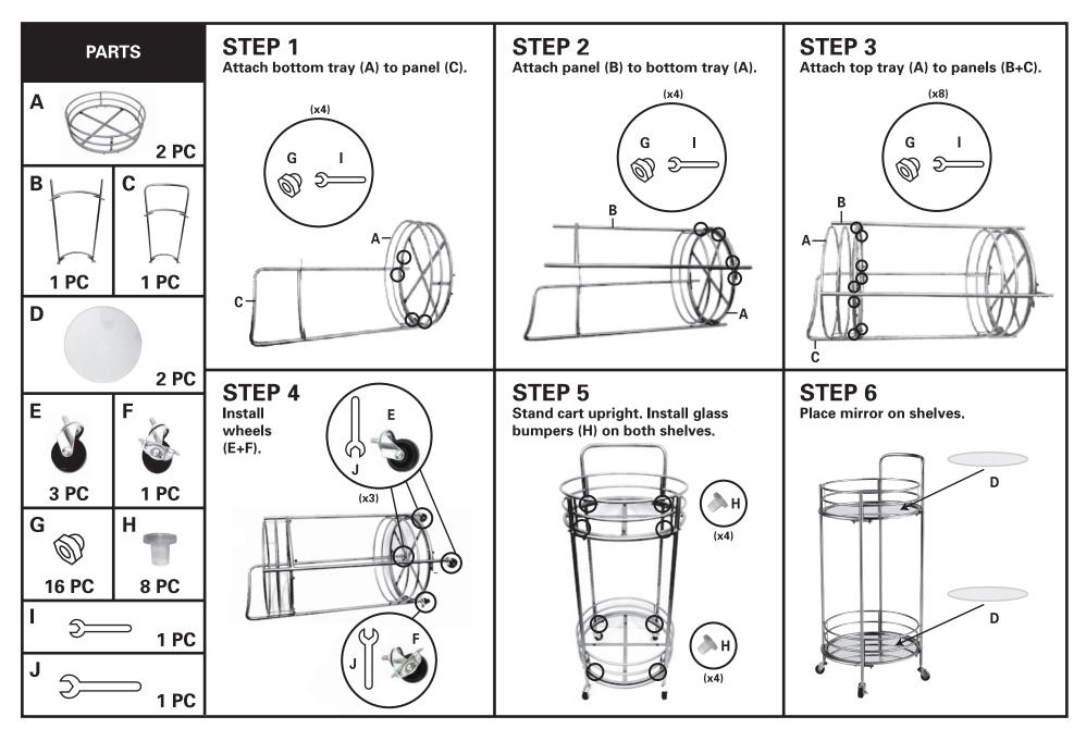
NOTE: Cap nuts (G) will be attached to the bottom of both shelves (A). Please remove before assembly.
