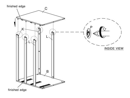
Attach the Top Panel (A) to the Left & Right Side Panel (B & C) and Top Support Rail (K) and tighten the Minifix Cam Lock (P) with screwdriver (not provided).
