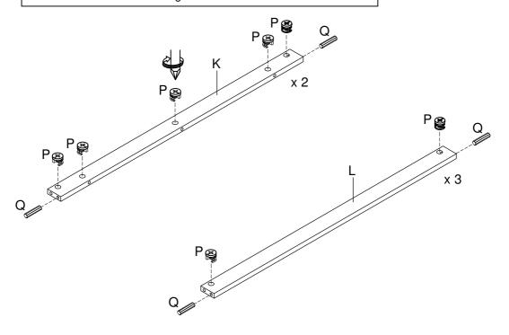
Attach the Top & Center Support Rail (K & L) to the Left Side Panel (B) and tighten the Minifix Cam Lock (P) with screwdriver (not provided).
