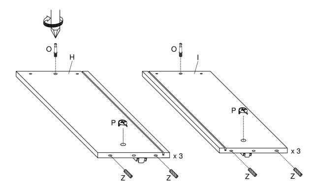
Insert Minifix Cam Bolt (O), Minifix Cam Lock (P) and Wood Dowel (Z) to the Drawer Back Panel (F) with screwdriver (not provided) as shown. Then insert Minifix Cam Lock (P) to the Drawer Bottom Support Rail (J).
