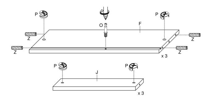
Attach the Drawer Left & Right Side Panel (H & I) to the Drawer Back Panel (F) and tighten the Minifix Cam Lock (P) with screwdriver (not provided).
