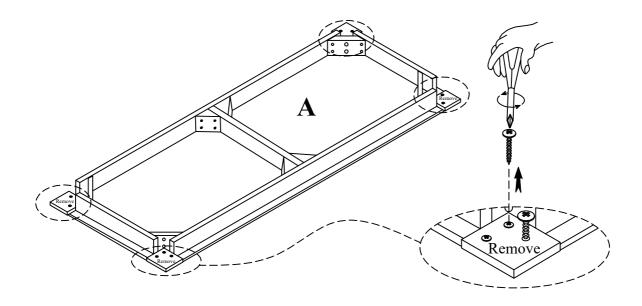
2 Place the Bench Top (A) upside down on the floor with a piece of cloth or carpet underneath to prevent from scratching. Attach the Bench Leg (B) to the Bench Top (A) using Flat Washer (C), Lock Washer (D) and Hex Nut (E) with Wrench (F). Do not fully tighten until all nuts and bolts are attached.
