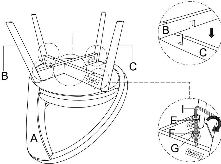
Take the Allen Key, and turn the bolts until the legs are secured. **DO NOT TIGHTEN COMPLETELY.** Stop when you feel you are adding force to tighten the bolt.
