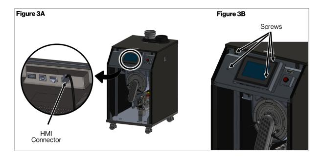
7. Remove the HMI assembly from the boiler cabinet (Figure 4). Be careful not to drop the HMI assembly.
