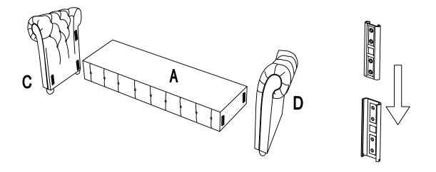
Hook on the Back Frame (B) to Left Panel (C) & Right Panel (D) properly.
