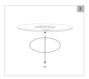
Insert the Flush Mount baseplate alignment bolt into the 1/8" hole and center the base receiver hole with the 2-1/8" hole.
