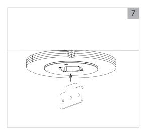
Once hand tight use the provided Pillar Mount tool to tighten the shims and mounting nut so the pillar is secure in place.
