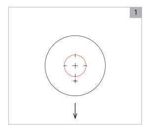
Print the provided template on page 4. Position the center of the template at the desired location for the center of the Pillar Mount. Make sure the small 1/8" mark is facing toward the front of where the Piller Mount will be facing.
