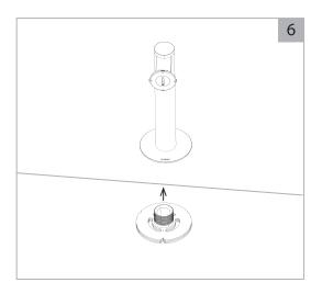
Insert the mounting nut with shims into the pillar hole and start threading the mounting nut and shims by hand into the Pillar base.
