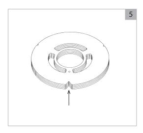
Ensure the V notch of all the shims are aligned for correct fitment of the mounting hardware
