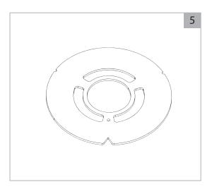
Provided are depth shims to accommodate a large range of surface thickness'. Use the appropriate amount of shims to ensure a tight fit of the mounting nut and the pillar base. The Flush Mount kit has a minimum mounting surface thickness of 7/8" (22mm) and a Maximum of 1-9/16" (40mm)
