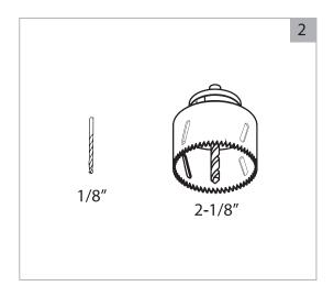
Use a 2-1/8" hole saw to cut a hole in the surface for the mounting nut Using the template as a center guide. Use a 1/8" drill bit to drill a hole for the alignment bolt on the FlushMount base.
