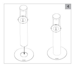
Place the pillar onto the base temporarily to verify alignment is correct.
