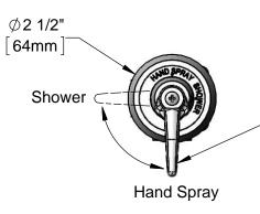
Rotate Lever Handle 1/4 Turn Between Shower or Hand Spray Positions. Handle Points to Indicator Markings on Escutcheon.
