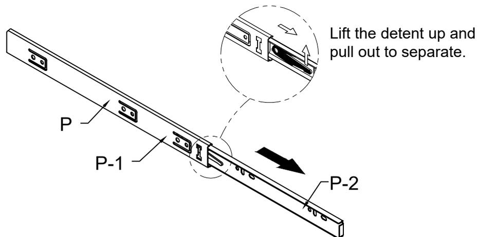
**7** Attach the first part of Slide Rail (P) to Center Panel (D) and Right Panel (E) by using Bolts (S), and tighten with Screwdriver (AE).
