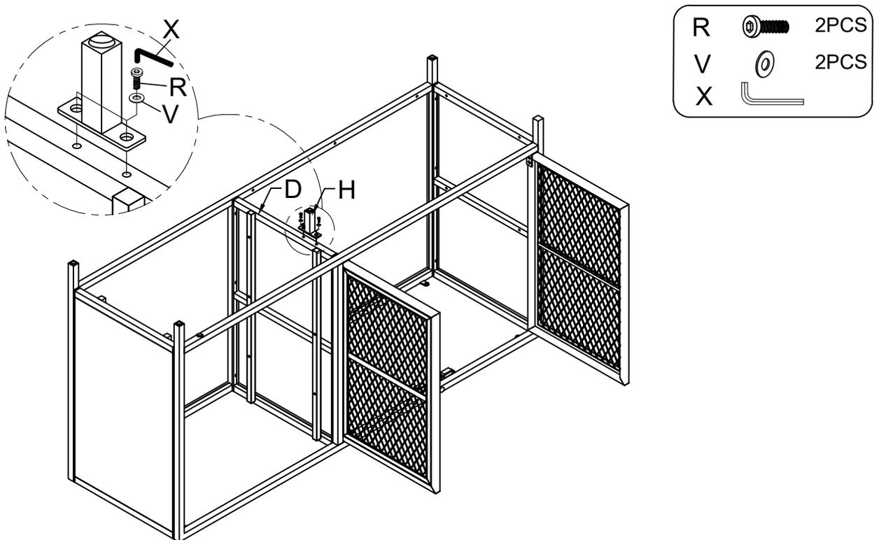
**3** Attach the Front Frame (A) and Back Frame (B) to Top Panel (N) by using Bolts (R), Flat Washer (V), and tighten with Allen Key (X).
