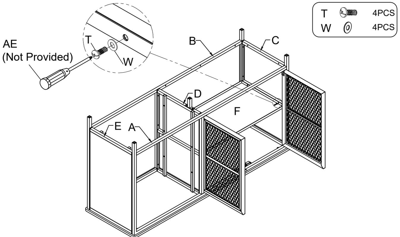
**5** Attach the Bottom Panel (G) to Left Panel (C) and Center Panel (D) by using Bolts (T), Flat Washer (W), and tighten with Screwdriver (AE).
