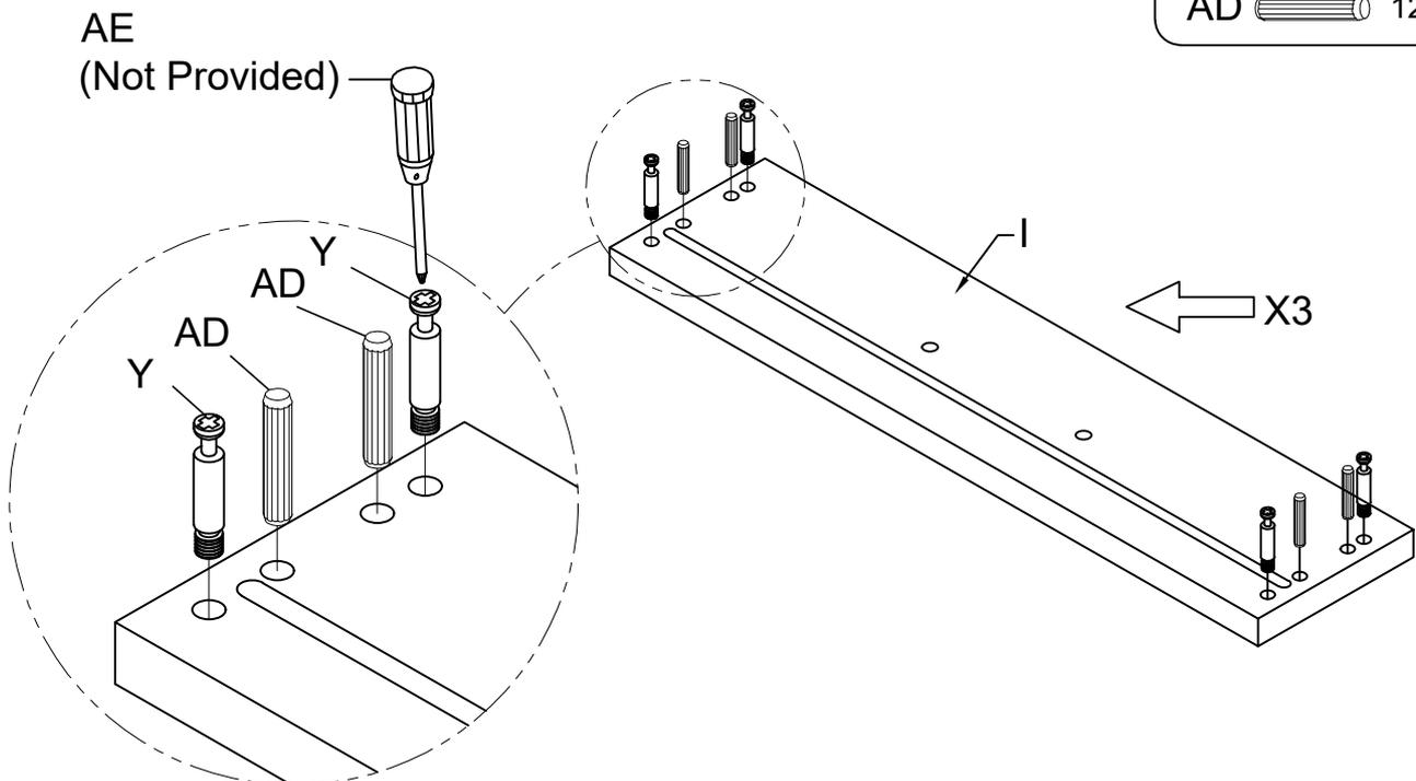
**9** Attach the Drawers Side - Left (J) and Drawers Side - Right (K) to Drawers Front (I) by using Nut (AC), and tighten with Screwdriver (AE).
