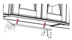
1. Center the fixture in the mounting space. Measure 1/2" from each end of fixture for mounting clip placement. Use screws to secure clip to mounting surface.
