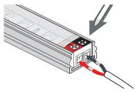
2. Insert stripped wires from power supply or receiver into outer terminals, Red wire to (+ or DC12V) side marked in red, Black wire to (- or GND) side of tape marked in black; tighten screws.
