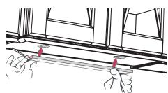
2. Snap fixture into mounting clips.
