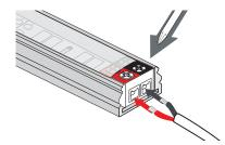
2. Insert stripped wires from power supply or receiver into outer terminals, Red wire to (WW+) side marked in red, Black wire to (CW-) side of tape marked in black; tighten screws.
