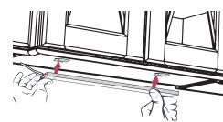
2. Snap fixture into mounting clips.
