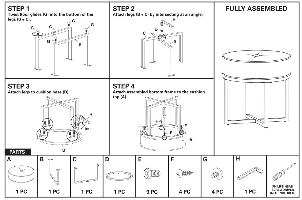
NOTE: PHILIPS HEAD SCREW DRIVER REQUIRED FOR ASSEMBLY (NOT INCLUDED)
