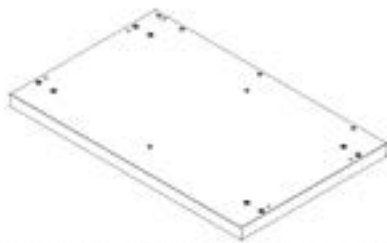
F3 SINK CABINET FLOOR PANEL ASSEMBLY - A4M03560 (x1) 37 3/16"x23 3/8"x2 5/8" (66x594x944)
