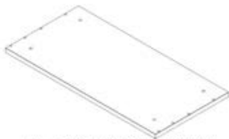
T8 TABLETOP PANEL - A4M03625 (x1) 47 7/8"x23 3/8"x1 1/4" (32x593x1216)
