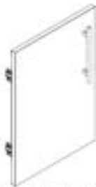
D1 PIZZA OVEN CABINET DOOR ASSEMBLY L - A4M03546 (x1) 28 7/16"x19 5/8"x15/16" (24x498x722.5)
