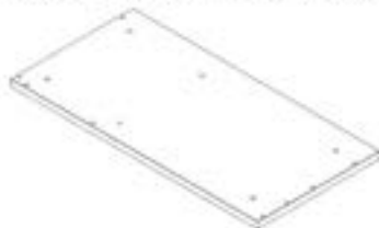
T9 TABLETOP PANEL ASSEMBLY - A4M03639 (x1) 47 3/16"x23 3/8"x1 1/4" (32x593x1199)
