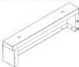
T5 PIZZA OVEN CABINET MARBLE PANEL ASSEMBLY L - A4M03549 (x1) 24 1/8"x4 5/16"x6 3/4" (109x172.2x612)
