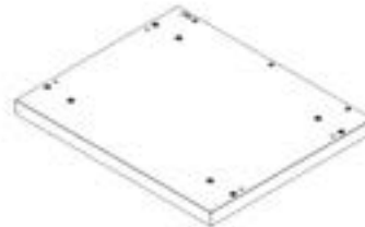
F4 FRIDGE CABINET FLOOR PANEL ASSEMBLY - A4M03595 (x1) 28 1/8"x23 3/8"x2 5/8" (66x594x715)
