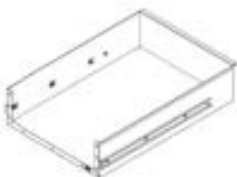
D12 DRAWER BODY ASSEMBLY - A4M03621 (x2) 22 1/4"x15 13/16"x4 15/16" (126x402x565)
