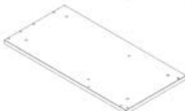
T6 TABLETOP PANEL ASSEMBLY - A4M03615 (x1) 47 3/16"x23 3/8"x1 1/4" (32x593x1199)
