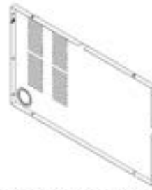
G10 GRILL CABINET BACK PANEL ASSEMBLY - A4M03055 (x1) 1 3/16"x22 7/8"x38 3/16" (30x581x970)
