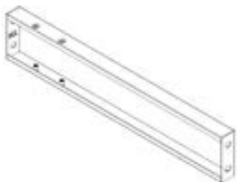
H7 HORIZONTAL CHANNEL ASSEMBLY - A4M03623 (x2) 16 5/16"x2 15/16"x1" (25x75x414)
