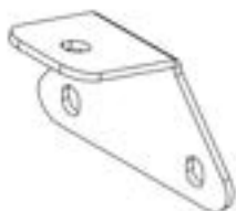
J5 RAFTER BRACKET - A4M03803 (x3) 3 5/8"x2 11/16"x2 1/16" (52x68x91.5)
