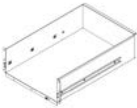
D4 SINK CABINET DRAWER BODY ASSEMBLY - A4M03571 (x1) 22 1/4"x16 1/16"x6 7/16" (164.2x408.4x565.4)
