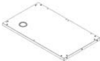
T1 PIZZA OVEN CABINET TABLETOP ASSEMBLY - A4M03543 (x1) 40 3/16"x23 3/8"x1 1/4" (32x594x1020)
