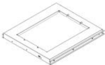
H3 TRASH CAN BRACKET ASSEMBLY - A4M03610 (x1) 18 1/16"x15 13/16"x (35x401.60x458)
