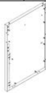
S3 SINK CABINET SIDE PANEL ASSEMBLY L - A4M03562 (x1) 33 3/8"x23 3/8"x1 3/8" (35.00x594.00x848.20)
