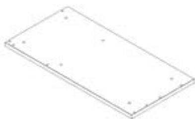
T9 TABLETOP PANEL ASSEMBLY - A4M03639 (x1) 47 3/16"x23 3/8"x1 1/4" 1 1/4" (32x593x1199)
