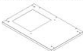
T4 SINK CABINET TABLETOP FRAME - A4M03566 (x1) 37 3/16"x24 1/8"x1 1/4" (32x612x944)
