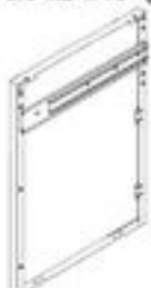
S9 SIDE PANEL ASSEMBLY - A4M03638 (x1) 33 3/8"x23 3/8"x1 15/16" (50x594x848.2)
