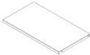
L4 SHELF ASSEMBLY - A4M03644 (x2) 27 3/4"x15 7/16"x1" (25x392.2x705)
