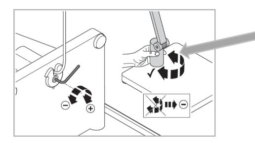
3. Attention. Please just tighten the screw "D" only so tight that you can move the base easily with just 2 fingers.
