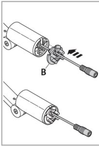
2. Place the Attenzia Task light on e.g. desk plate, then unscrew the existing metal bolt and locate the plastic part "B". Lead the cable of the Task light through the aperture of the base plate "A". In the last step put the second plastic part "C" from the bottom side of the base plate "A" and fix it with the screw "D".
