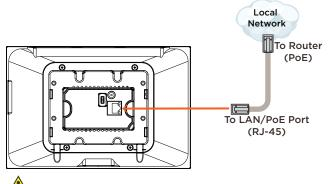
**IMPORTANT NOTE!** If a PoE network router is not available, a PoE network injector can be used.
