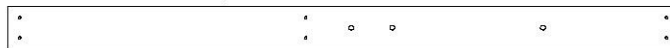
M03 | PLANCHE DE MUR - W4L13944 (x1) | 5/8 po x 3 3/8 po x 52 3/8 po (16 x 86 x 1 332)
