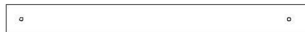
M04 | RAIL MURAL - W4L13946 (x2) | 5/8 po x 3 3/8 po x 34 1/8 po (16 x 86 x 868)
