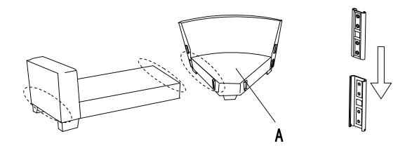
Then hook on Middle Seat Frame to Left and Right Corner Seat (A) properly. (Middle Seat Frame is not in the Corner Seat carton)
