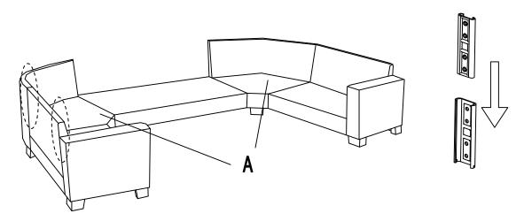
Then hook on Middle Back Frame to Left and Right Corner Seat (A) properly. (Middle Back Frame is not in the Corner Seat carton)
