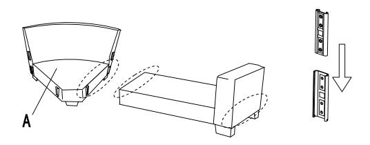
Hook on Left Seat Frame to Left Panel and Corner Seat Frame (A) properly. (Left Seat Frame is not in the Corner carton)
