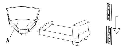
Then hook on Left Seat Frame to Left Panel and Corner Seat (A) properly. (Left Seat Frame is not in the Corner Seat carton)
