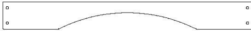
L5 | GUÍA DE PARED DE LA CASA CLUB - W4L14567 (x1) | 5/8"x4 3/8"x40 3/8" (16x112x1024)
