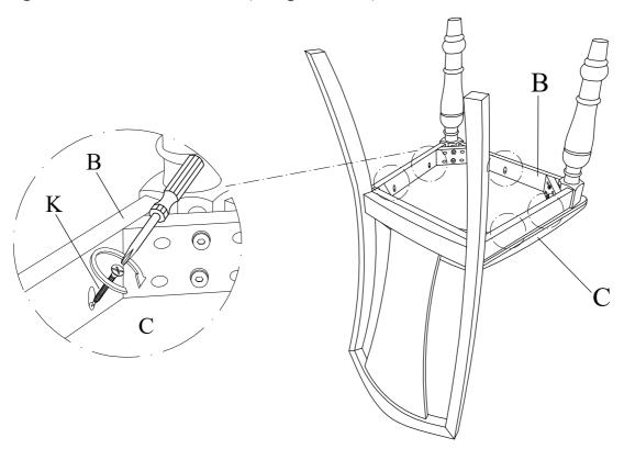
4 Stand chair up on an even surface and check that it is balanced. If there is a slight wobble, apply downward pressure in the corner where a leg is uneven. Keeping pressure in that corner, tighten all bolts. If balanced, apply downward pressure evenly in the center and tighten all bolts. Do not over-tighten beyond hole depth.
