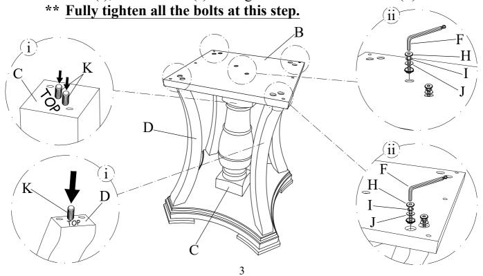
Place Table Top (A) upside down on a soft surface. Align and attach Mounting Plate (B) to Table Top (A) using JCBC Bolt (H), Lock Washer (I), Flat Washer (J) and tighten with Allen Wrench (F). Screw in the Leveler (L) to the Bottom Base (E).
