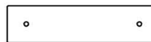
M25 | SUPPORT DE TABLE - W4L16037 (x2) 5/8 po x 3 3/8 po x 13 1/2 po (16 x 86 x 342)
