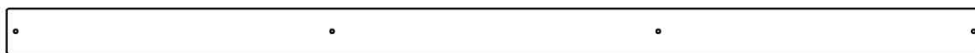
N01 | PLANCHE DE PLANCHER - W4L16076 (x1) 5/8 po x 2 3/8 po x 50 7/8 po (16 x 60 x 1292)
