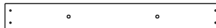
H10 | PLANCHE DE FIXATION - W4L16045 (x1) | 1 po x 3 3/8 po x 27 7/8 po (24 x 86 x 707)
