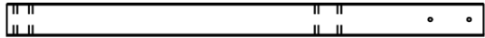
SP50 | SUPPORT DE POUTRE DE BALANÇOIRE - W4L16085 (x1) 3 3/8 po x 3 3/8 po x 49 3/8 po (86 x 86 x 1254)
