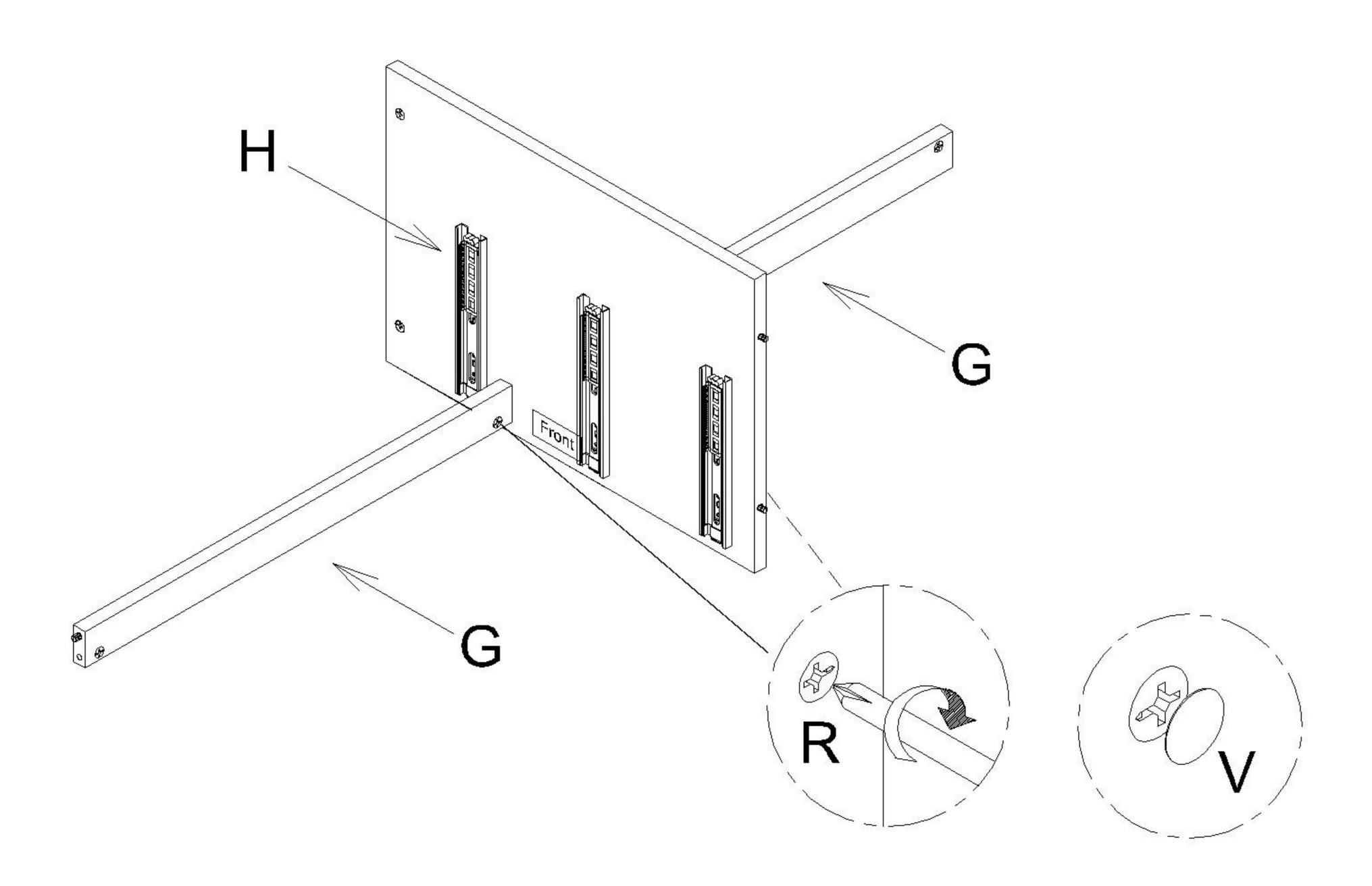
Attach Left & Right Side Panel (B & C) to Center Bar (G) and secure with the Cam Lock (R) attached in the Step 3. Cover Cam Lock (R) with Cam Lock Cover (V).
