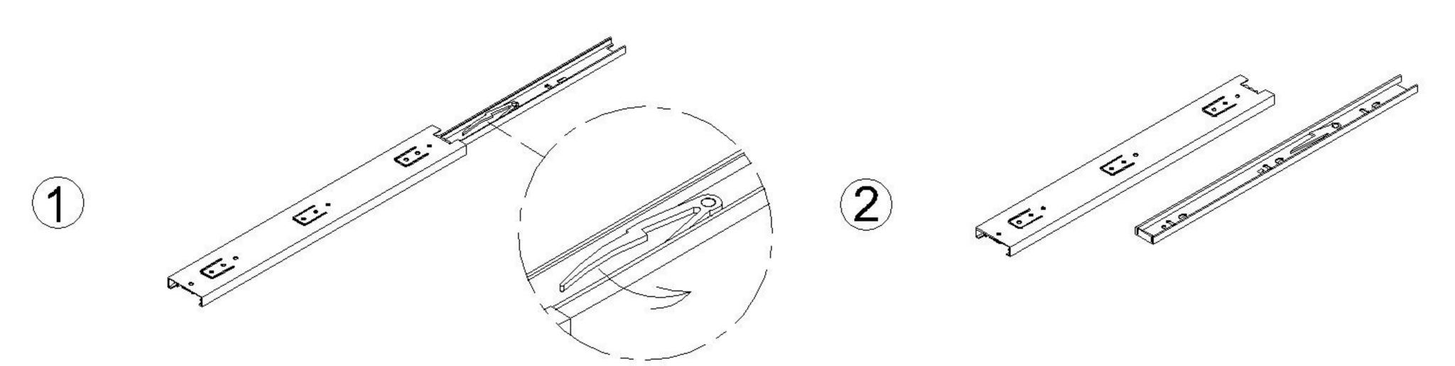
Disassembled the Runner (U) to 2 parts. Fix 1 part on the Left & Right Side Panel (B & C) and fix the other part on the Left & Right Drawer Side (J & M).
