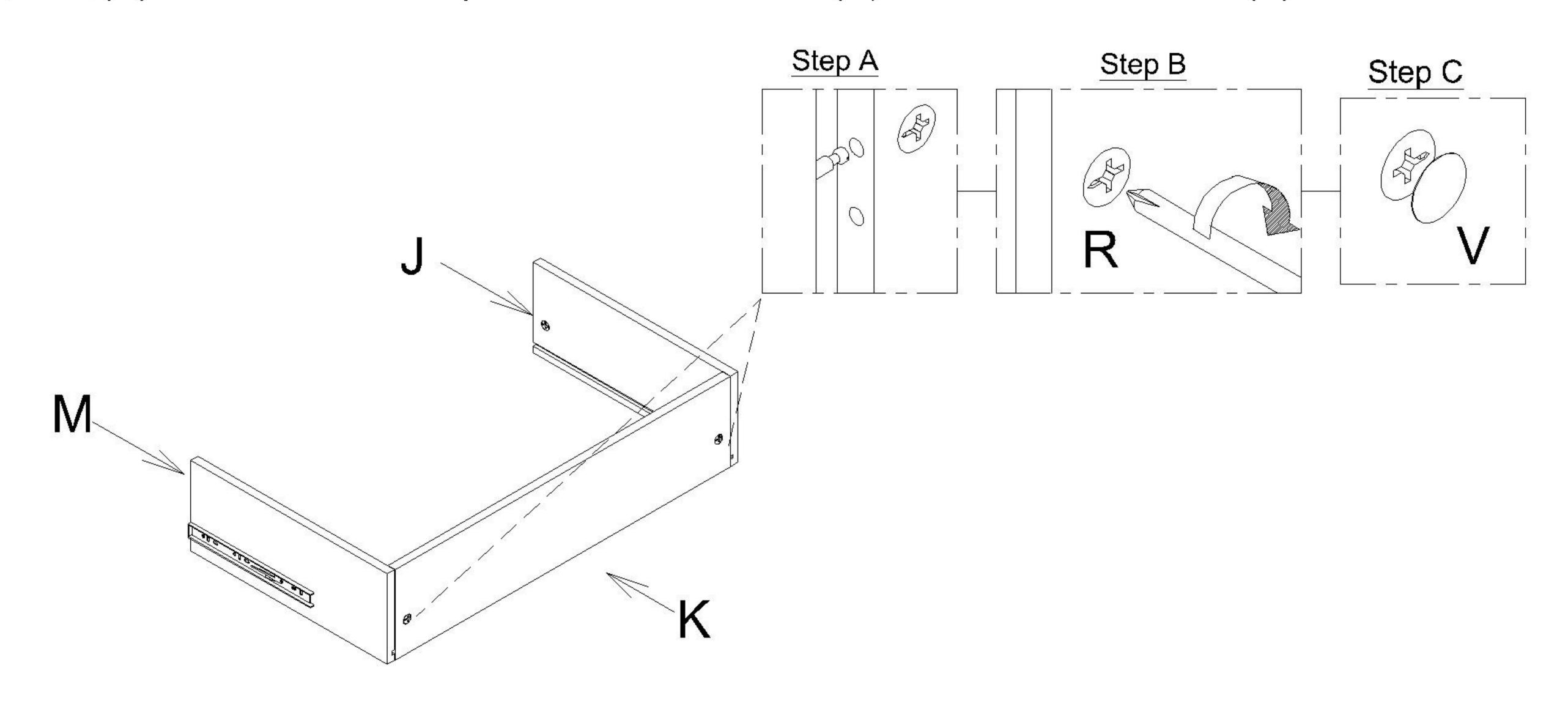
Slot in Drawer Base (L) in corresponding grooves. Attach Left & Right Drawer Front (I & N) to Drawer Box and secure with Cam Lock (R) attached in the Step 14. Cover Cam Lock (R) with Cam Lock Cover (V).
