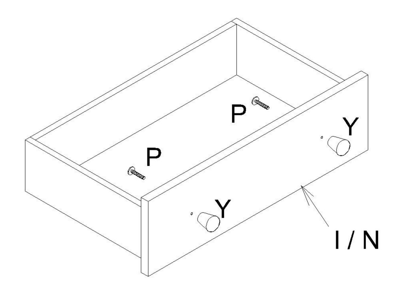
18 Stand the assembled unit up. Slot Drawers into assembled unit.
