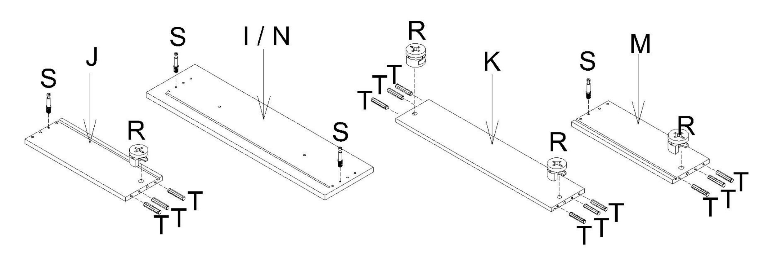
Attach Left & Right Drawer Side (J & M) to Drawer Back (K) and secure with Cam Lock (R) attached in the Step 14. Cover Cam Lock (R) with Cam Lock Cover (V).
