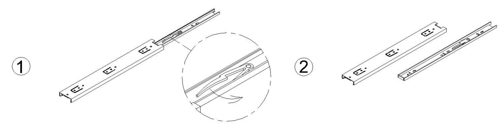
Disassembled the Runner (U) to 2 parts. Fix 1 part on the Partition (H), and fix the other part on the Left & Right Drawer Side (J & M).
