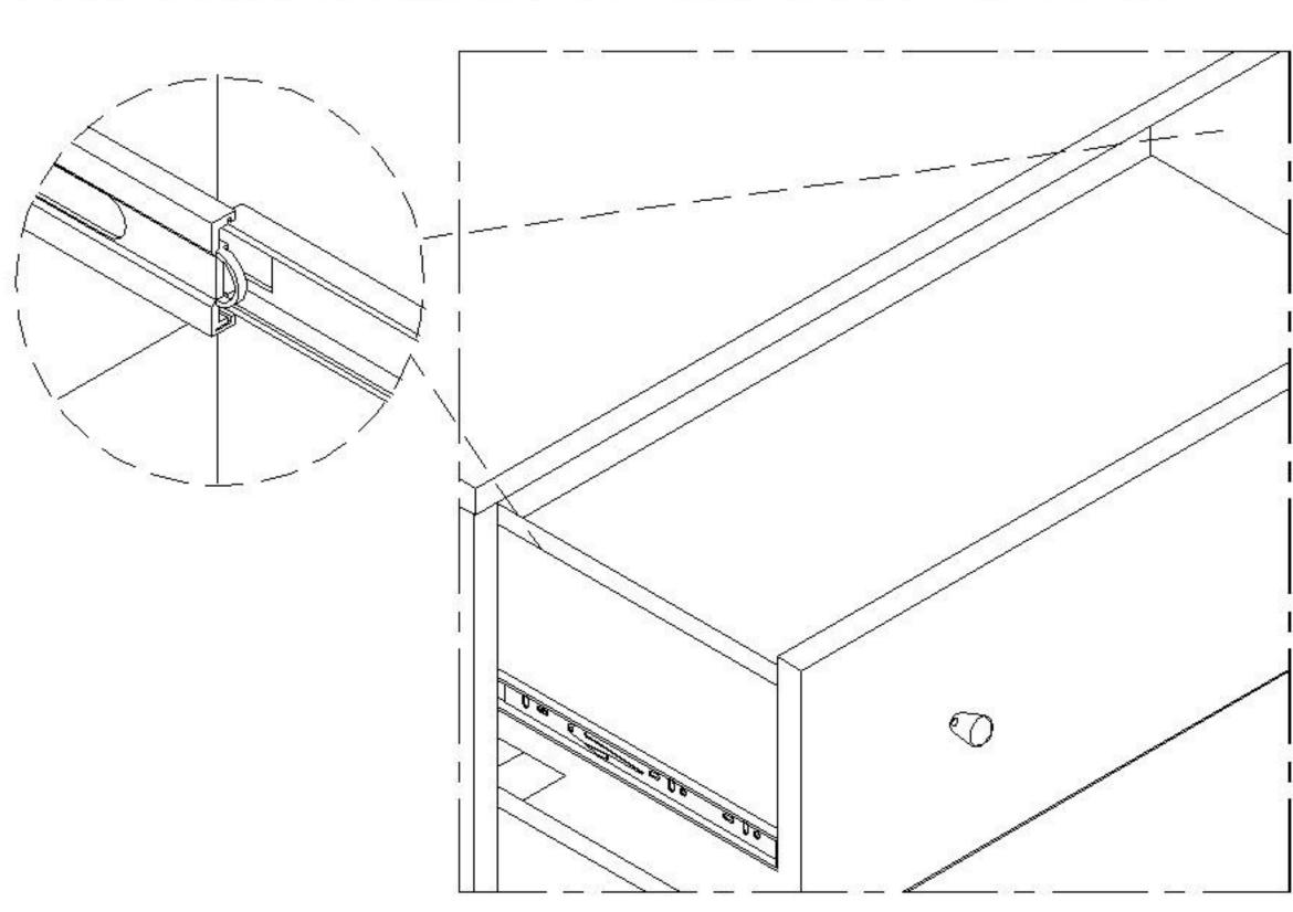
NOTE: Align and pull/push the triggers on both sides of drawer box into the metal track on interior side of side panel.
