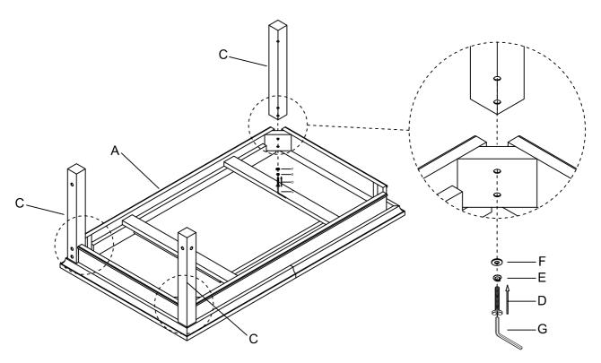
Attach Bottom Shelf (B) to 3pcs Metal Leg (C) using Bolt (D), Spring Washer (E) and Flat Washer (F) by Wrench (G). Then attach the 4th Metal Leg (C) to both Bottom Shelf (B) and Top Panel (A) by the same method. Finally attach Caster (H) to the Bottom Shelf (B) by using Screw (I) with Screwdriver
