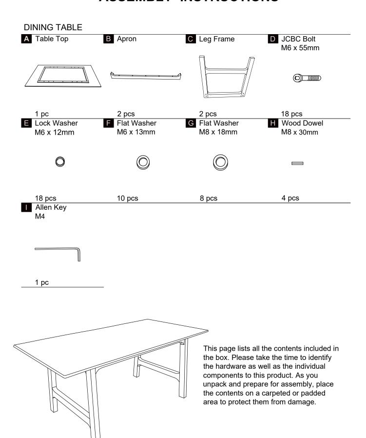
Place the Table Top (A) on a protective surface. Insert Wood Dowel (H) into the Apron (B). Then, attach the Apron (B) to the Table Top (A) using JCBC Bolt (D), Lock Washer (E) and Flat Washer (F) with the Allen Key (I).
