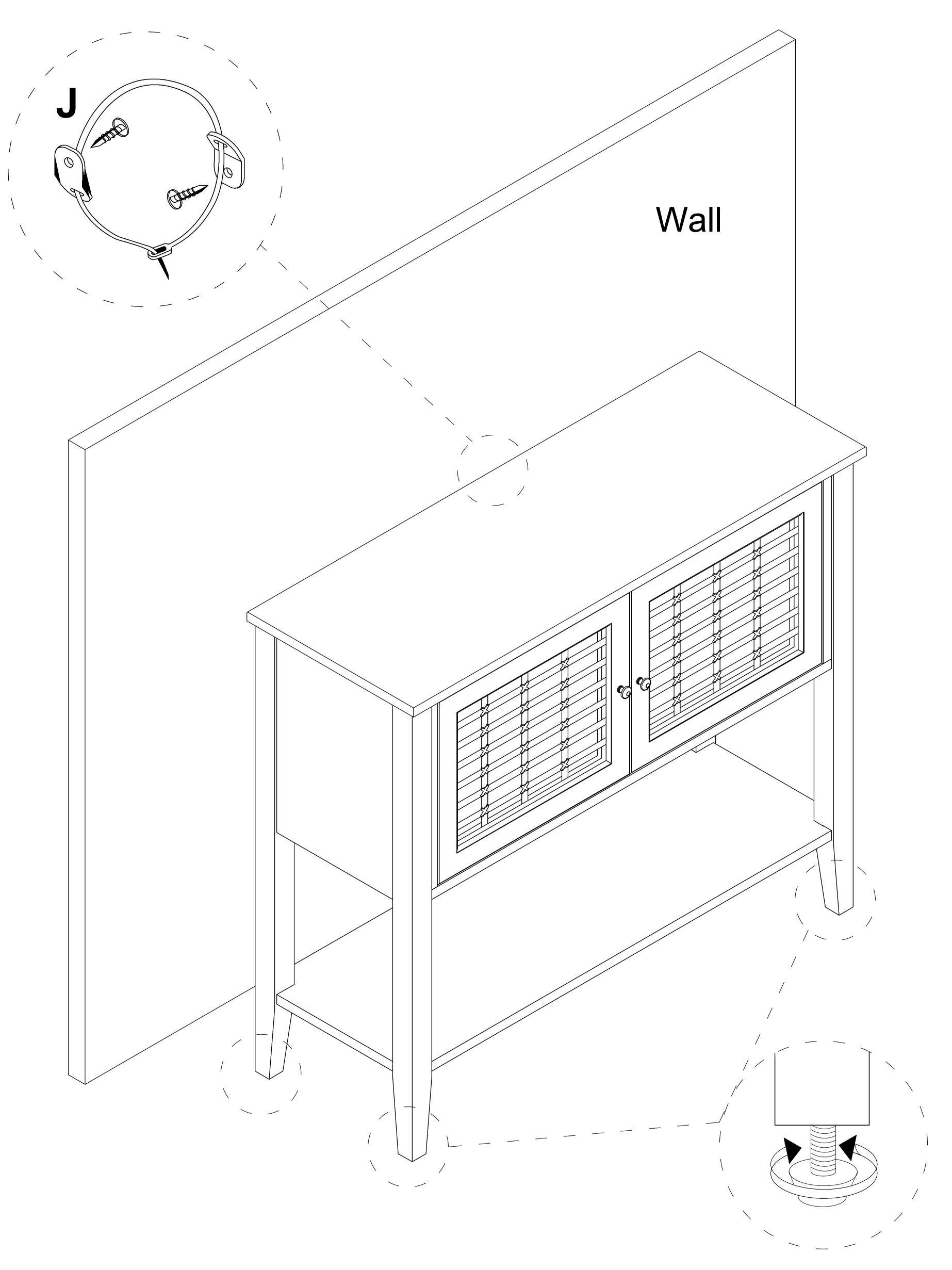
Turn left or turn right to adjust the leveler until the server is stabilized.
