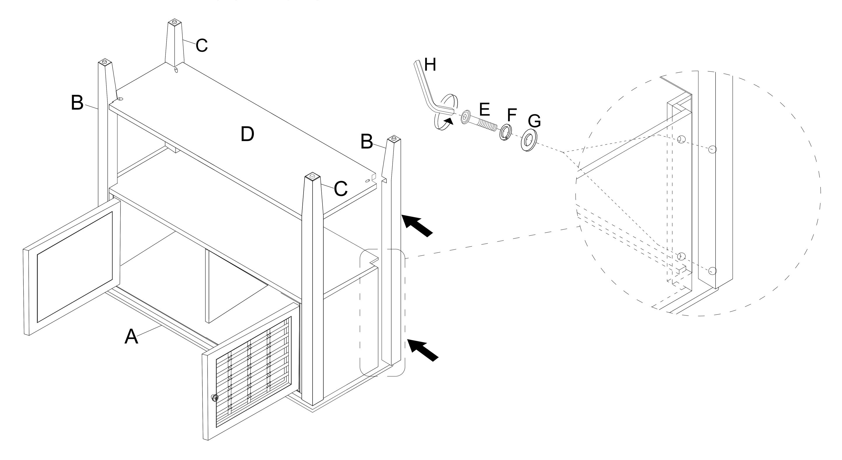
Fix Shelf (D) to Leg (B & C) using Wood Screw (I) with Screwdriver (Not Provided).
