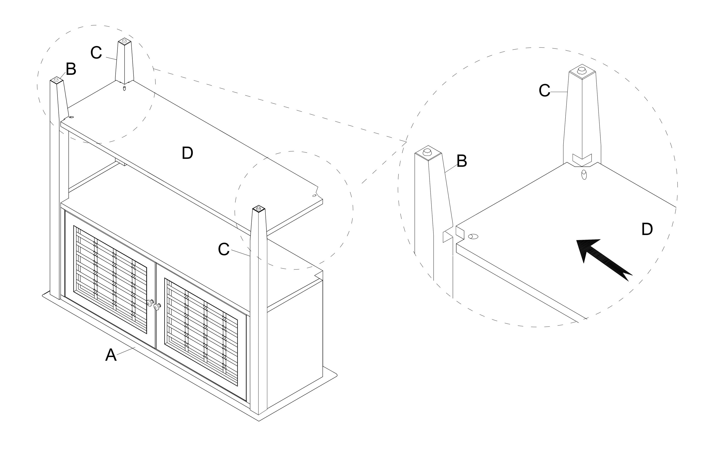
Attach Leg (B) to Server Top (A) using Bolt (E), Spring Washer (F) and Flat Washer (G) with Allen Wrench (H). Fully tighten all the bolts in this step.
