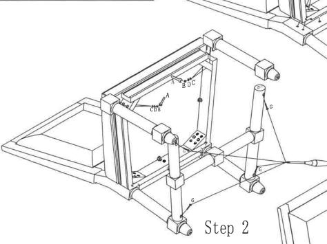
Assemble the chair on soft and clean surface to prevent scratching. Loosen screws holding upholstered seat to seat apron assembly, it's not necessary to remove the seat completely.
