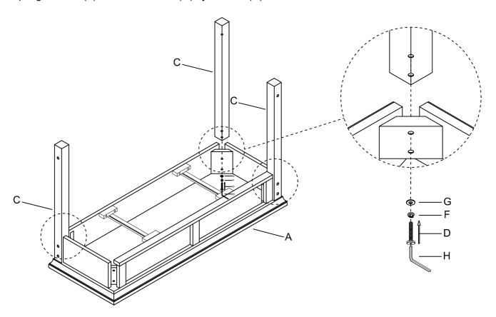
Attach the Bottom Shelf (B) to the 3pcs Metal Leg (C) using Bolt-Small (E), Spring Washer (F), Flat Washer (G) and Iron Bracket (I) by Wrench (H). Then attach the 4th Metal Leg (C) to both Bottom Shelf (B) and Top Panel (A) by the same method. Finally lock them up to 100%.
