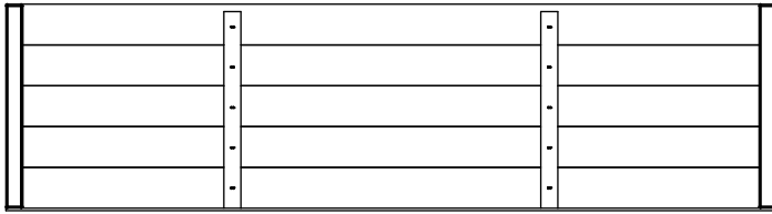
(1) RP3 - ROOF PANEL - W2A01862 1 3/8"x16 1/8"x59 1/2" (35x410x1532)
