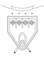
4 If you use the sliders, you can mount the speaker cables to the terminal at this point. If you use the mounting points, it is easier to install the speaker first and mount the cable to the terminal after the speaker is mounted to the wall.
