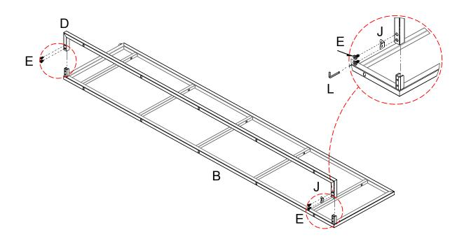
Attach Mounting Plate (J) to the Back Frame (D) and Side Frame - LSF (C) with Bolt (E) and Allen Wrench (L), making sure the Mounting Plate (J) extend DOWNWARD as shown.
