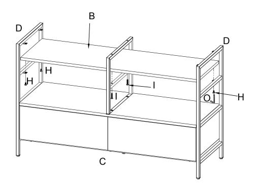
Attach Top Panel (A) to the Side Frame (D) and Center Frame (E) by using Bolt (H), Bolt (I) and Allen Wrench (O) as shown.
