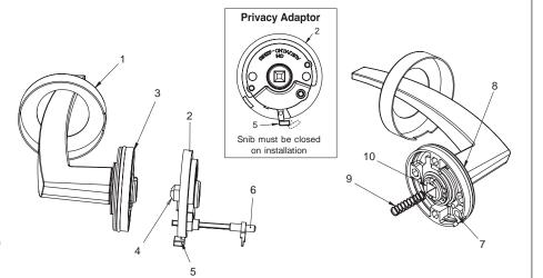
NOTE: Carefully follow these instructions when installing. Screws to be tightened to a recommended 2.5Nm torque.
