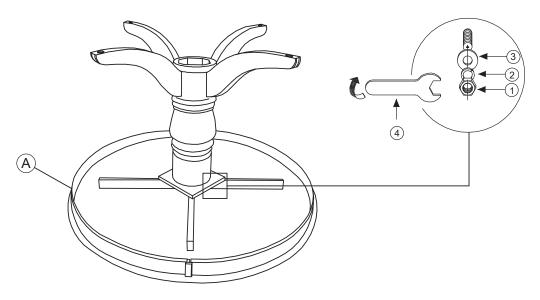
Turn the assembled table to the upright position carefully. Make sure the table is level, and then securely tighten all nuts at this stage. Assembly is now completed.
