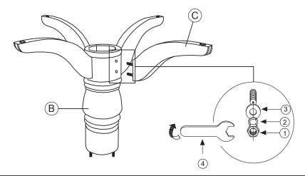
Place Table Top (A) face down on a clean and flat soft surface to prevert from being scratched. Insert Hanger Bolt of Oxtogen Coloum (B) into the predrilled holes of Mounting Plate at table top (A), then tighten with Flat Washer (3), Spring Washer (2) and Hex Nut (1) with Wrench (4).
