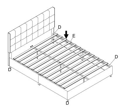
Insert the Bolt (R) to Slat (E) and Rail Section (D), then turn the Ratchet Tool (U) to tighten them.
