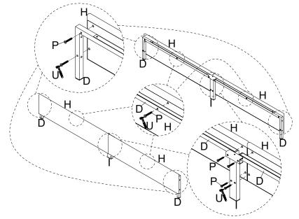
Cover the Fabric Cover (L) to the assembled headboard. Attach the Lower Headboard (B) and Footboard (C) to Rail Section (D), insert Bolt (P), turn the Ratchet Tool (U) to tighten them.
