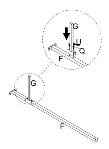
Attach the Center Rail - Front / Rear (F) to the Lower Headboard (B) and the Footboard (C), insert the Bolt (Q), turn the Ratchet Tool (U) to tighten them.
