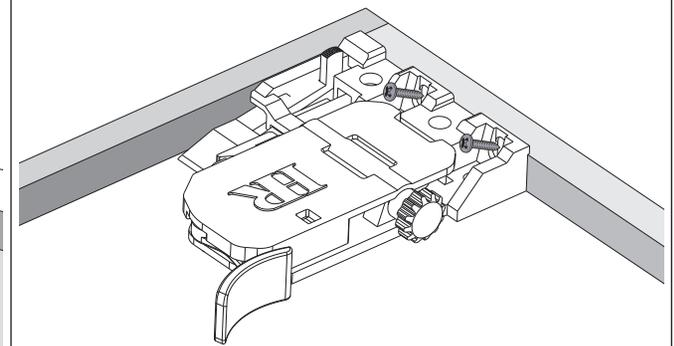
Turn drawer box upside down and drill holes for undermount slide release clips. Shown with optional multi-tool (HR-TOOL-300)
