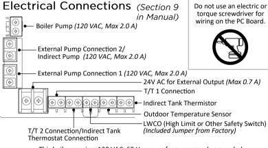
This boiler requires 120 VAC, 60 Hz power from a properly grounded circuit. Use caution when connecting power to the boiler
