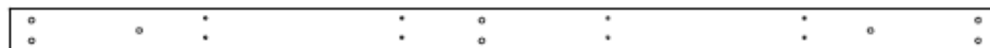
H03 SUPPORT DE PLANCHER - W4L22139 (x1) 1 po x 3 3/8 po x 74 5/8 po (24 x 86 x 1894)
