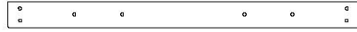
H06 SUPPORT DE PLANCHER - W4L22143 (x1) 1 po x 3 3/8 po x 45 1/8 po (24 x 86 x 1147)
