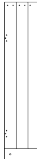
WP11 PANNEAU MURAL - W2A05004 (x1) 2 1/16 po x 10 3/16 po x 45 9/16 po (52 x 258 x 1158)
