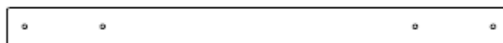
H01 SUPPORT DE PLANCHER - W4L22142 (x1) 1 po x 3 3/8 po x 45 1/8 po (24 x 86 x 1147)
