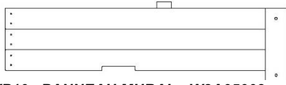
WP10 PANNEAU MURAL - W2A05003 (x1) 2 1/16 po x 13 5/16 po x 45 5/8 po (52 x 338 x 1158)
