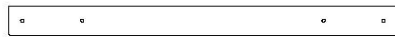
H01 SUPPORT DE PLANCHER - W4L22142 (x1) 1 po x 3 3/8 po x 45 1/8 po (24 x 86 x 1147)
