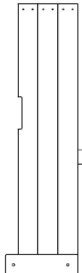
WP10 PANNEAU MURAL - W2A05003 (x1) 2 1/16 po x 13 5/16 po x 45 5/8 po (52 x 338 x 1158)
