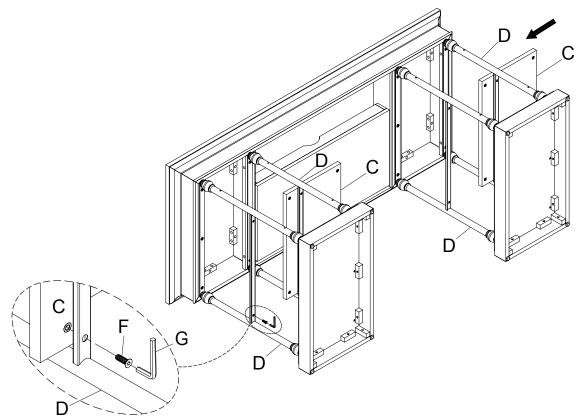
Assembly the Cross Bar (E) onto the Side Frame (D) and using the Bolt (F) by Allen Wrench (G).
