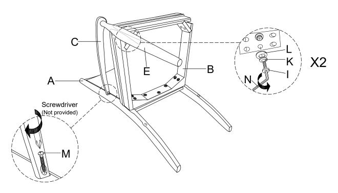
Attach the Right Front Leg (F) to the Cushion Seat (B) using JCBC Bolt (I), Lock Washer (K) and Flat Washer (L) with the Allen Key (N). Then, attach the Right Arm (D) to the Back Frame (A) using Wood Screw (M) with a screwdriver (not provided).
