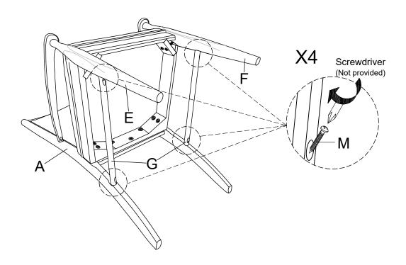
Stand the chair on an even surface and check for balance. If the chair wobbles slightly, apply downward pressure on the uneven leg and tighten the bolts to correct the imbalance. Once the chair is balanced, apply downward pressure evenly in the center of the chair and tighten all bolts, being careful not to over-tighten beyond the hole depth.
