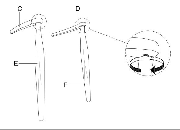
Attach the Left Front Leg (E) to the Cushion Seat (B) using JCBC Bolt (I), Lock Washer (K) and Flat Washer (L) with the Allen Key (N). Then, attach the Left Arm (C) to the Back Frame (A) using Wood Screw (M) with a screwdriver (not provided).
