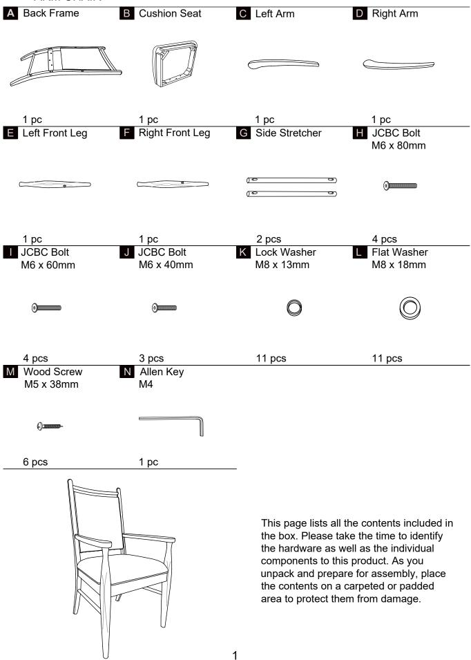
Place the Back Frame (A) on a protective surface. Attach the Cushion Seat (B) to the Back Frame (A) using JCBC Bolt (J), Lock Washer (K) and Flat Washer (L) into the middle holes, and using JCBC Bolt (H), Lock Washer (K) and Flat Washer (L) into the corner holes, tightening with the Allen Key (N).
