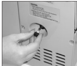
Figure 10. Replacing the fuse located underneath motor housing.
