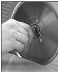
Figure 7. Turn the screw clockwise for blade removal.
