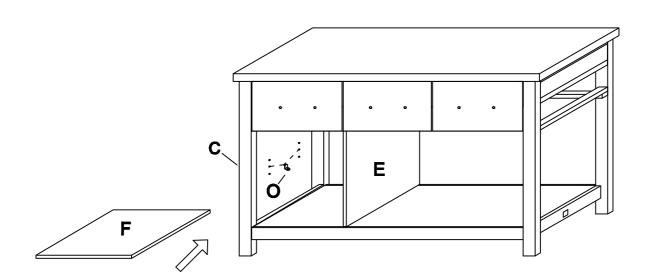
\*\*\* Do not tighten screws & bolts until the entire unit is completely assembled.
