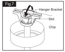
Hang the fan on hanger bracket, and rotate the downrod until the chip on the hanger bracket snaps into the slot on the hanger ball. Note: For sloped ceiling installation, make sure the slot of hanger ball and the chip of hanger bracket face down.
