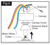
Slide canopy, canopy cover (Making sure the smooth side of canopy cover is facing downward.) and downrod stand cover onto downrod as shown, then thread motor wires through downrod.
