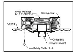
Turn OFF the electric circuit at the Tighten the hanger bracket to the outlet box with two mounting screws and washers. (Make sure the outlet box is securely installed so that it will be able to support the fan weight.) Attach the safety cable hook to the ceiling, and make sure the safety cable hook is covered by the fan canopy.
