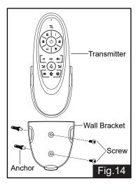
Install the transmitter wall bracket on the wall with two anchors and two screws and place transmitter in it carefully.
