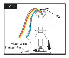
Loosen the collar screws out part way. Insert the downrod into the collar. Slide hanger pin through holes of collar and downrod.
