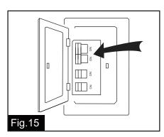
Turn ON the electric power at the main fuse or circuit breaker box.
