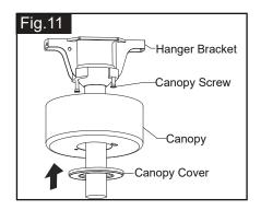
Slide the canopy up to ceiling and over the two canopy screws on hanger bracket. Rotate canopy clockwise, next, while holding the canopy with one hand slide the canopy cover over the screws and rotate clockwise until tight.
