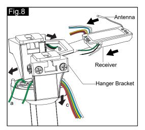
Move ground wires (a), outlet box wires (b), and motor wires (c) away from the center of the hanger bracket as shown.
