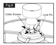
Tighten the two collar screws. Slide lock pin into hanger pin until it is locked into position.
