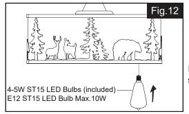
Install LED bulbs (included). See relamping label at socket area or packaging for maximum wattage allowed.
