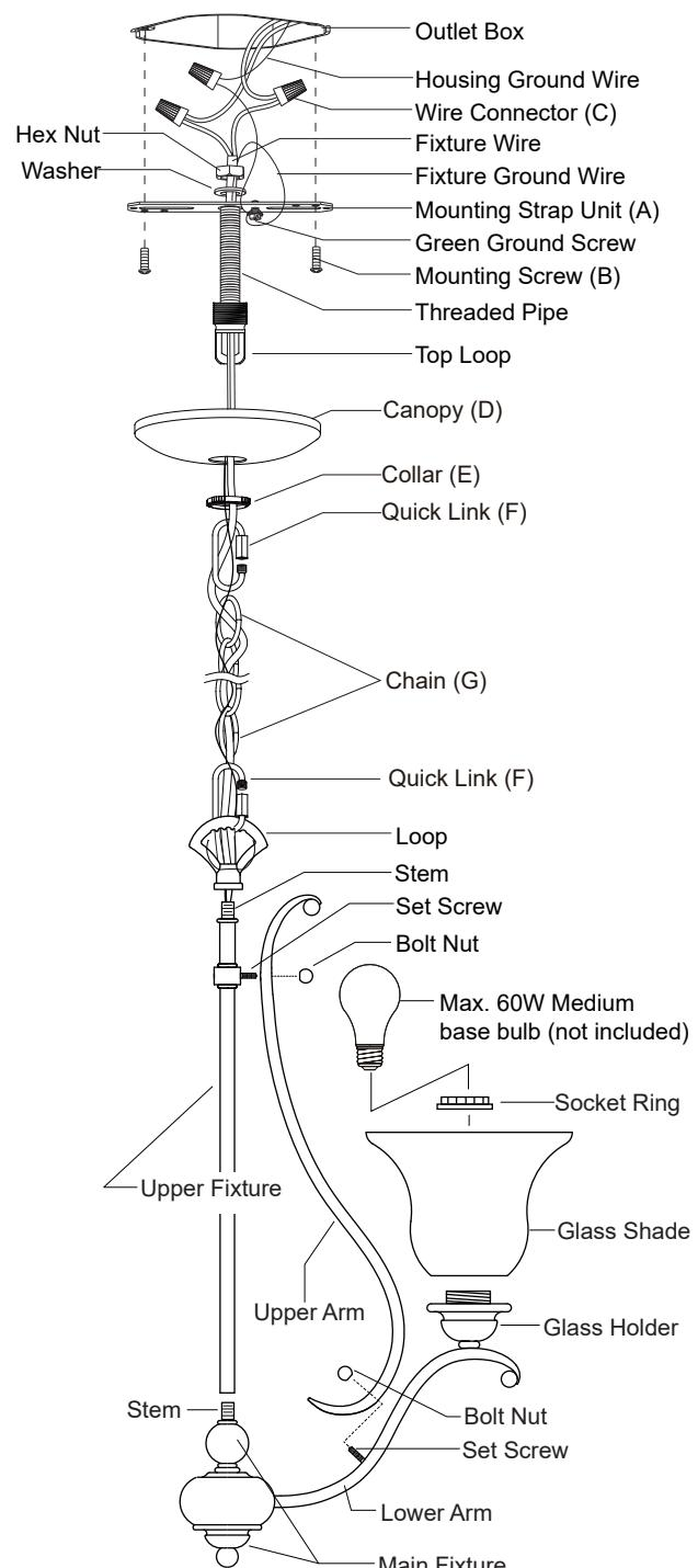
10. Attach the canopy (D) to the mounting strap unit (A) by inserting the top loop, then secure it with the collar (E).
