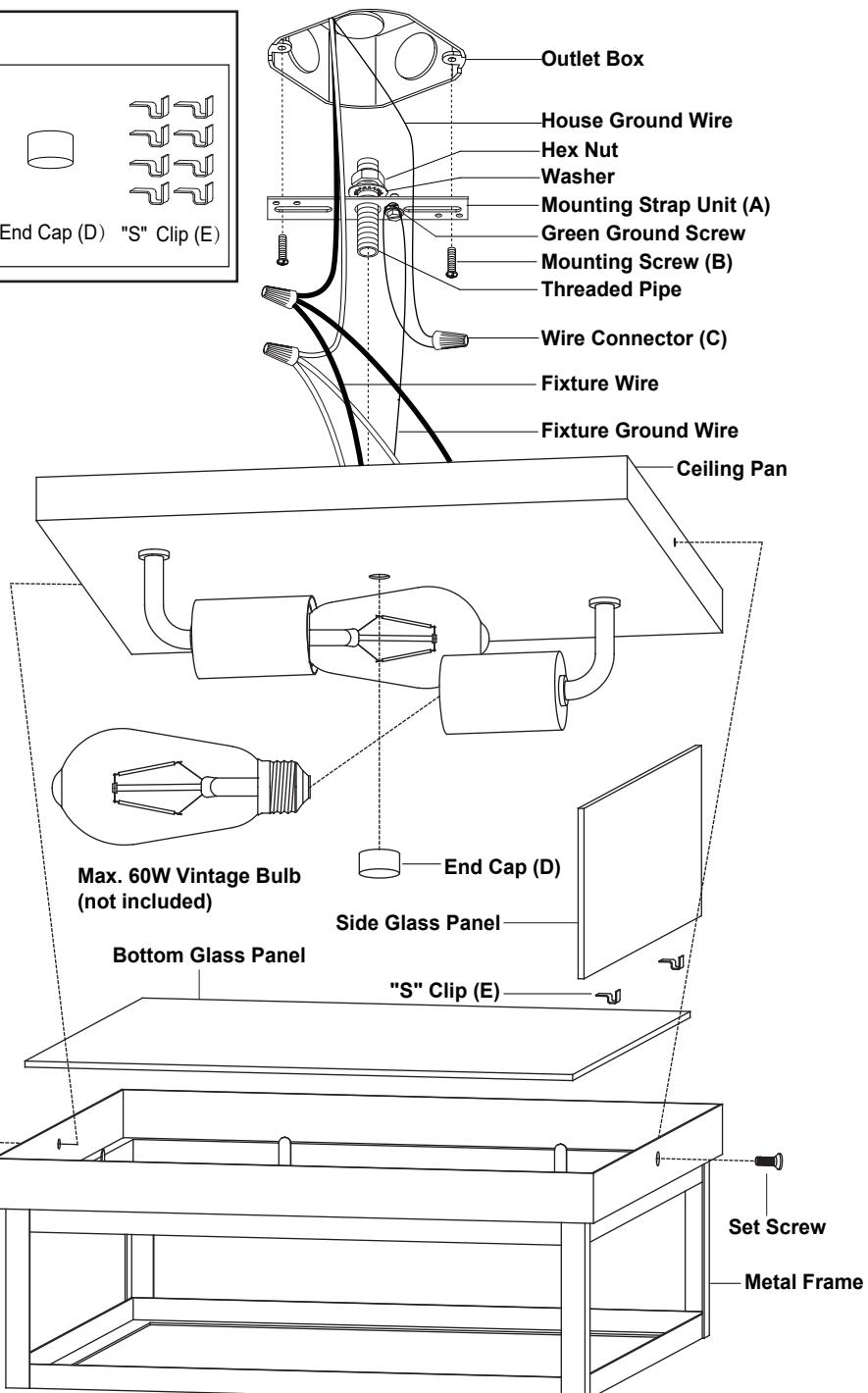
7. Place the bottom glass panel into the metal frame, and set the two "S" clips (E) each side on the slot and hold the bottom glass panel by inserting the side glass panels inside the metal frame. Then press the top clips on the fixture to secure the side glass panels.
