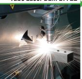
This is a complex machine that can cut and/ or etch designs into tubular and open shape products. The laser is not limited to holes, slots and/or straight end cuts. There is no hard tooling involved in running products so this opens up the possibilities of shorter runs that can be cost effective.
