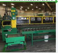
The Haven Tube Cutters are high-speed cutoffs that use a double cut process to re-cut tubing from mill lengths to customer-specified shorter lengths. With the Haven, there are no metal shavings to be removed after cutting. The end condition of the tubing after cutting is dimple-free with minimal burr.
