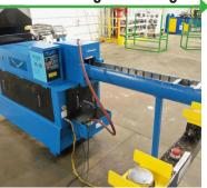
A ram swage is a fixed die that produces a smooth swage with no segment lines. The downside to a ram swage is that there is no adjustment in the tooling. If the wall thickness varies a little or if the O.D. is slightly larger or smaller, the fit of the swage will vary.
