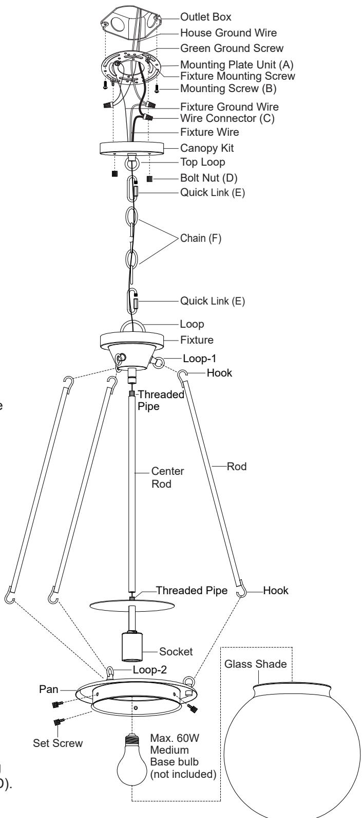
9. Attach the glass shade to the pan, then secure it with three set screws.
