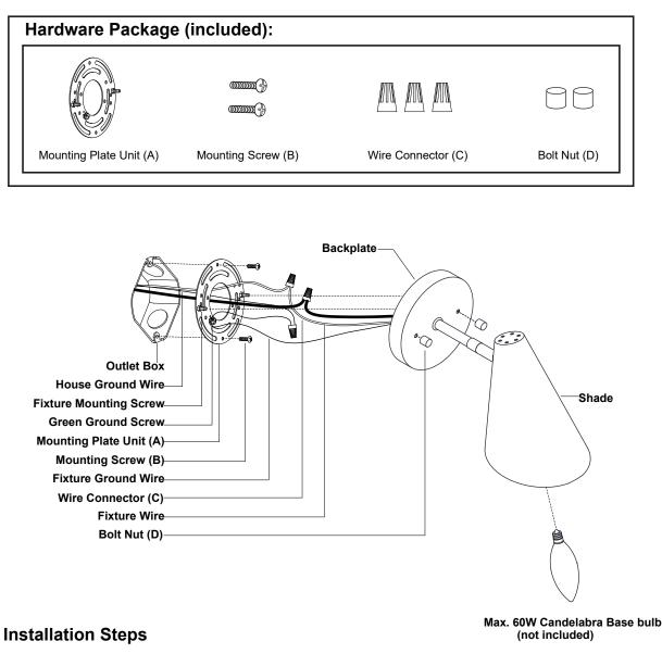
Turn off the power at fuse or circuit box.
