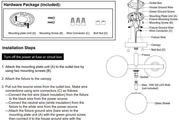
4. Attach the fixture to the mounting plate unit (A) by inserting the fixture mounting screws, then secure it with two bolt nuts (D).
