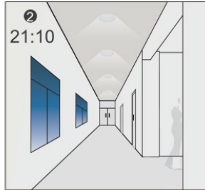
The light dims to stand-by level after the hold-time.
